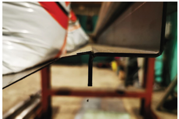
Figure 7 Static load test with sand bag ballast progressively applied until activation & opening
